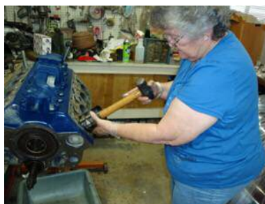
Installing pistons & connecting rod
