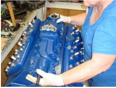
Installing intake manifold
