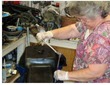
Installing oil pan
